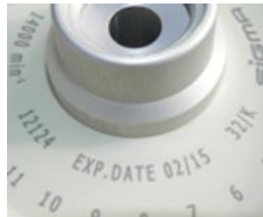
Fig. 7: Different service life – engraving on the bucket/rotor
