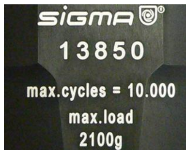
Fig. 7: Different service life – engraving on the bucket/rotor
