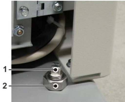
Fig. 8: Alignment at the front
